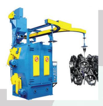
In the competitive world of today's industry, economical surface finishing is important. The ABSS range of Spinner Hanger Blast Machines are designed to handle the cleaning and surface preparation of typically awkward components that cannot be adapted to a Table or Tumble Blast Machines. Parts are loaded onto a hanger and rotated during the blast cycle for multiple angle cleaning.
