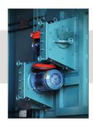
At the heart of the machine there are six (6) dynamically balanced ABSS Blast Turbines that generate the blasting curtain.
