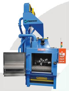
In the competitive world of today's industry, economical surface finishing is important. The ABSS range of Blast Machines offer a total solution to mass finishing, whether you need a single small machine or a complete system, the ABSS-GW range offer single load capacities of 75-1000kgs or more with system integration.
